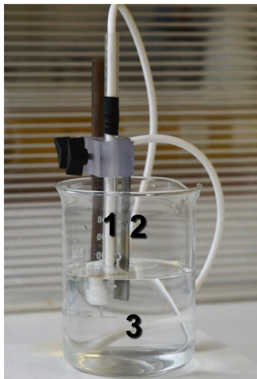
Figure 1 Experimental setup (left: scheme, right: photograph): 1 - main jet electrode, 2 - counter electrode, 3 - precursor solution, 4 - active plasma region
