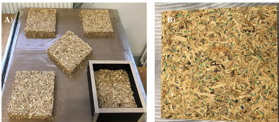
Fig.6. A) Manufacturing of the particleboards B) Particleboard with plasma treated PET flakes
